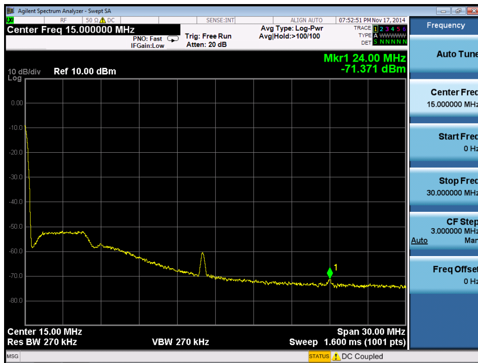
Figure 72. Spectrum of IF output without blocker present (signal -94dBm).
